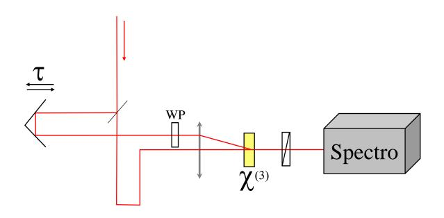
$$S(\tau,\omega) = \left| \int \mathcal{E}(t) |\mathcal{E}(t-\tau)|^2 \exp(i\omega t) dt \right|^2 \quad \text{Algorithme iteratif} \quad \phi(\omega)$$
