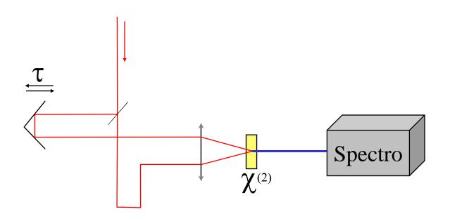
$$S(\tau,\omega) = \left| \int \mathcal{E}(t)\mathcal{E}(t-\tau) \exp(i\omega t) dt \right|^2 \qquad \text{Algorithme iteratif} \qquad \phi(\omega)$$
