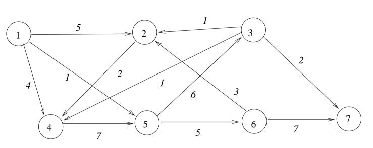
arc capacities as shown in italics: find the maximum flow between node s = 1 and t = 7
