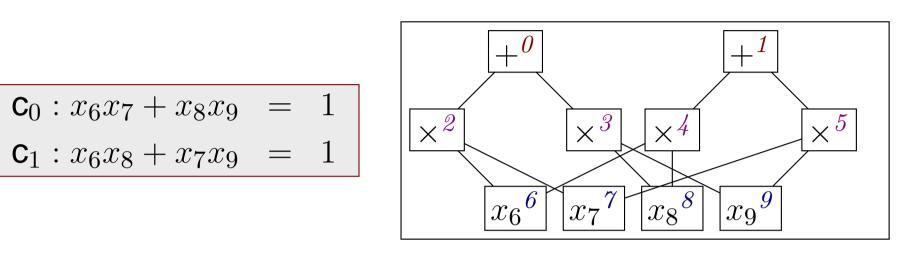
G<sub>DAG</sub> = group of automorphisms of expression DAG fixing: (a) root node set having same constr. direction and coeff. (constraint permutations), (b) operators with same label and rank and (c) leaf node set (variable permutations)
