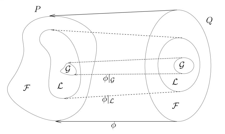
*Main idea*: if we find an optimum of Q, we can map it back to the same type of optimum of P, and for all optima of P, there is a corresponding optimum in Q. Also known as *exact reformulation*
