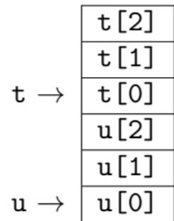
since `t` and `u` are (stack-allocated) arrays and arrays assignment is not possible
