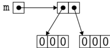
the integers being **immutable objects**, we can forget they are heap-allocated objects
