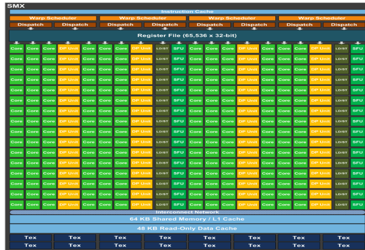
SMX: 192 single-precision CUDA cores, 64 double-precision units, 32 special function units (SFU), and 32 load/store units (LD/ST).
