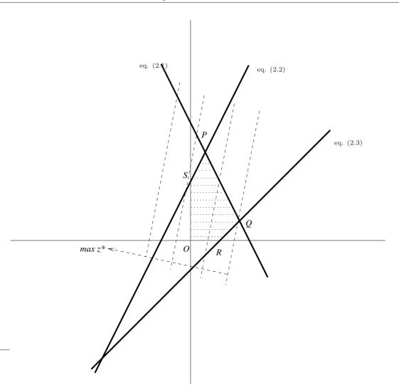
Figure 9.5: Objective function such that S is optimum.
