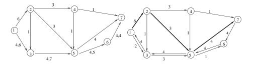
The next augmenting path is  $\{(1,2), (2,5), (5,7)\}$  with  $\beta = 3$ . The next flow has value  $\varphi = 4 + 3 = 7$ . The incremental network  $\bar{G}_2$  is shown on the right below.
