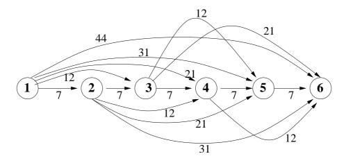
Any path from 1 to 6 represents a renewal plan; the cost of the path is the cost of the plan. We have to find a shortest path from node 1 to node 6. To this end we may either apply Dijkstra's algorithm
