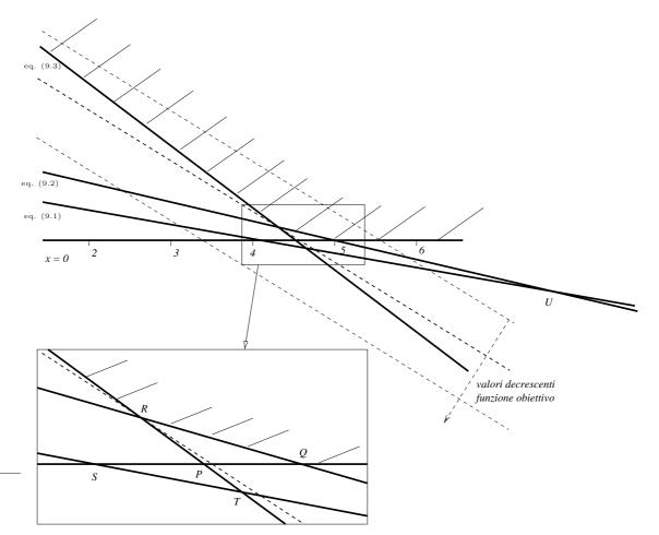
is evident from Fig. 9.2 that the optimal solution is at vertex R of the feasible polyhedron. Vertex
