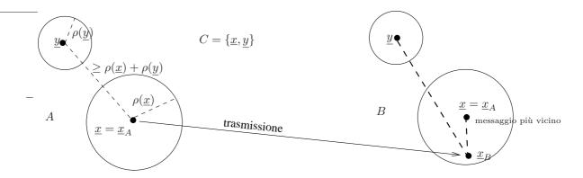
Formulate a (nonlinear) mathematical program to build an ECC C of 10 messages in  $\mathbb{R}^{12}$  (where all message components are in [0, 1]) so that the correction radius is maximized.
