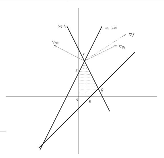
Figure 9.4: Optimality at P: the vector  $\nabla f$  is in the cone generated by  $\nabla g_1$  and  $\nabla g_2$ , where  $g_1(x) \leq 4$  is (2.1) and  $g_2(x) \leq 2$  is (2.2).
