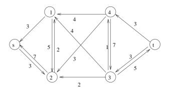
The graph exploration algorithm starting from s applied to the above graph finds  $S = \{s, 2, 1\}$ , so the cut with minimum capacity is given by arcs (i, j) with  $i \in S$  and  $j \in V \setminus S$ :
