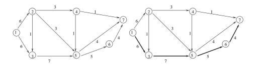
The augmenting path p in  $\overline{G}_0$  is  $\{(1,3), (3,5), (5,6), (6,7)\}$  with  $\beta(p) = 4$ . The new feasible flow has value  $\varphi = 0 + 4 = 4$ . The incremental network  $\overline{G}_1$  is shown on the right, below.
