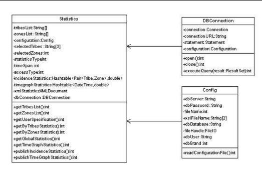
Figure 3: The UML class diagram for the user interface.
