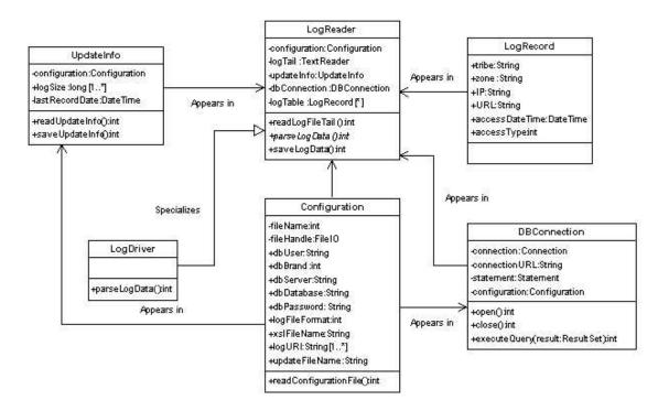
Figure 5: The UML class diagram for the log reading daemon.
