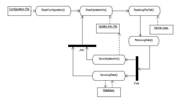
Figure 4: The UML activity diagram for the log reading daemon.
