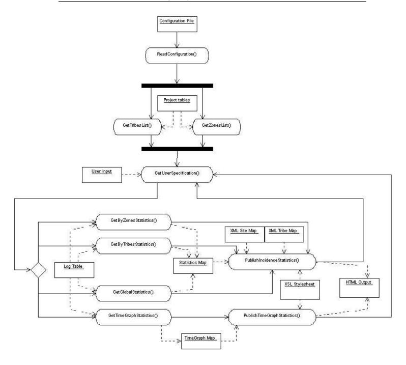
Figure 2: The UML activity diagram for the user interface.
